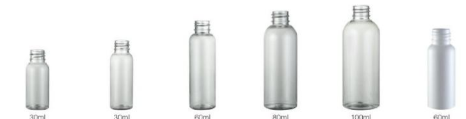
CT-L2030YA Ø20/410 W:6g H:68mm Dia.:28mm CT-L2030YB Ø20/410 W:8g H:79mm Dia.:28.5mm CT-L2060Y Ø20/410 W:10g H:102.5mm Dia.:32mm CT-L2080Y Ø20/410 W:8g H:101mm Dia.:36mm CT-L20100Y Ø20/410 W:10g H:107mm Dia.:40mm CT-L2460Y Ø24/410 W:12g H:94mm Dia.:35mm
